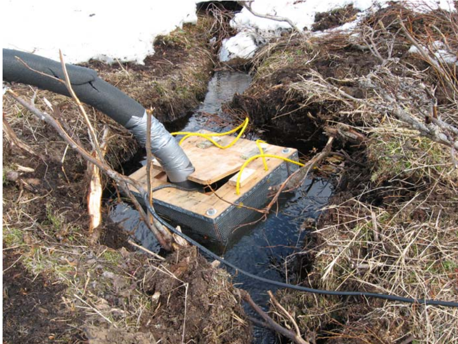
Figure 4. Water withdrawal point, drill rig number 1, Upper Talarik Creek Tributary. Screened intake was placed in an excavated site. Streamflow was observed immediately downstream of the intake in a 6 inch wide channel covered by vegetation.
