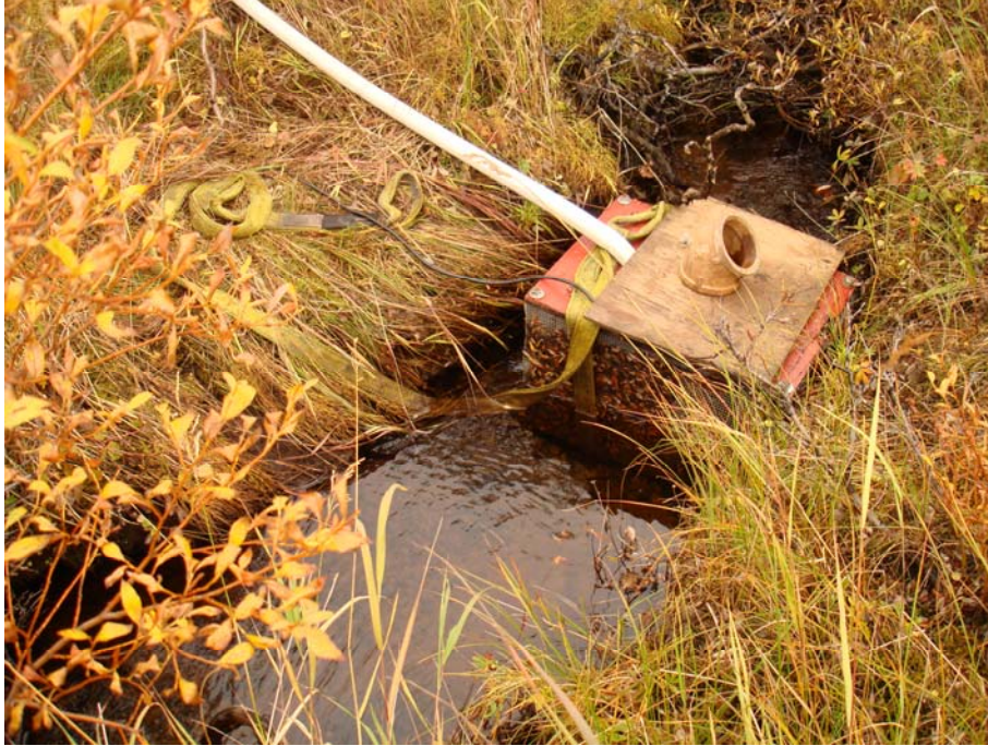
Figure 3. Water intake screen at water source for Drill Rig 1.
